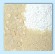
**Zinc Stearate CM -** this clear melt zinc stearate is one of the most widely used additives in the plastics field. It also serves as a lubricant or emulsifier in the toiletries and cosmetics areas, and can be used for mold release.
